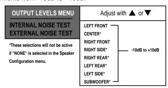
Using a Sound Pressure Level Meter such as Radio Shack model 33-2050 or 33-2055, set the weighting to C and the response to Slow. Adjust all output levels to achieve 75dB at the listening position.
